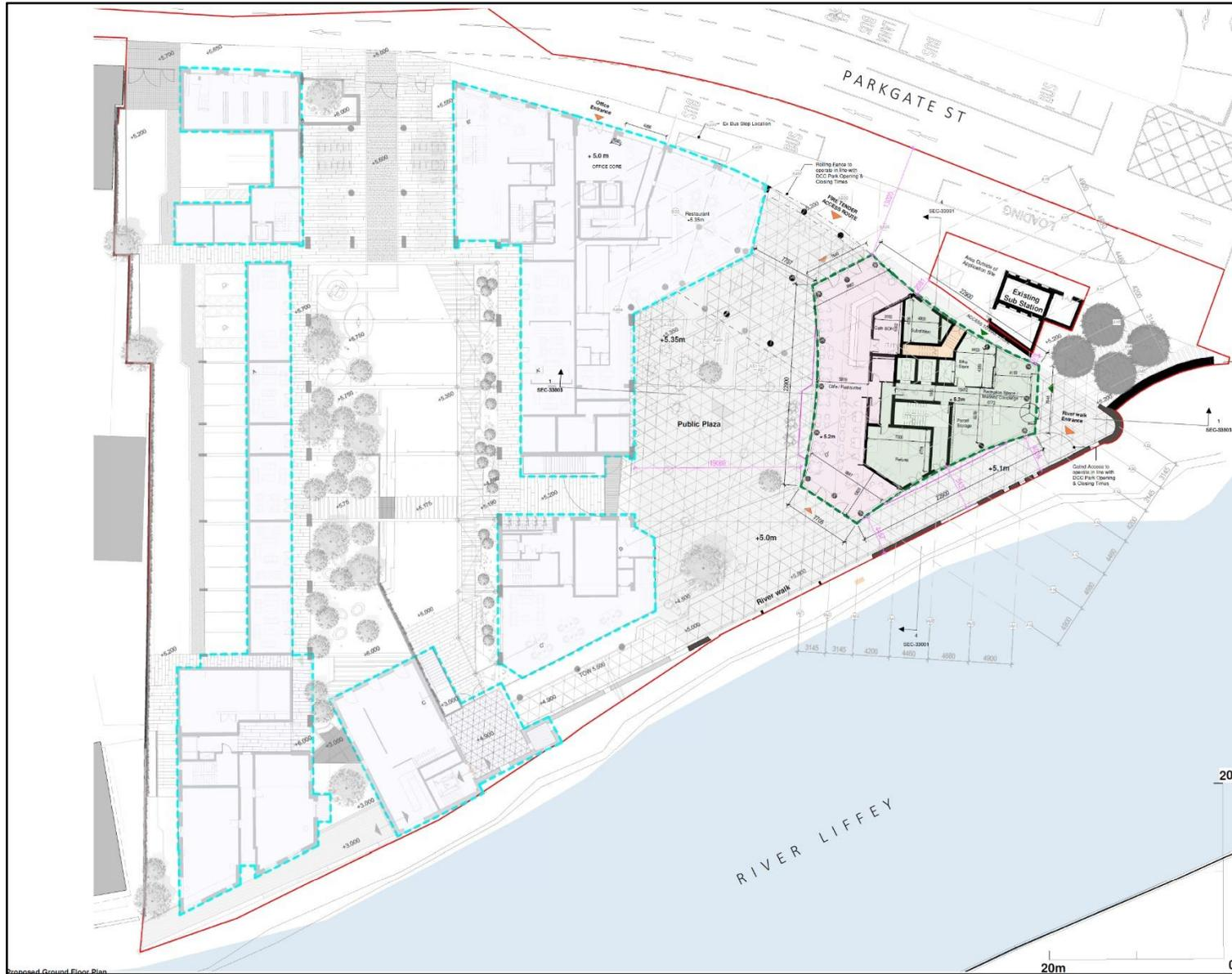
Figure 3. Ground floor layout the proposed development showing the Tower Building area within green dashed line.
